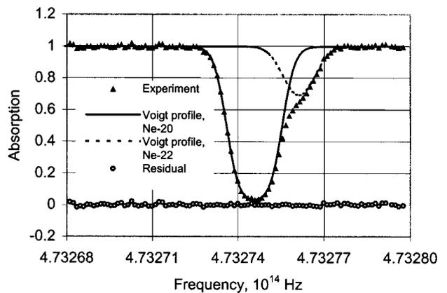
FIG. 2. Absorption spectrum for transition 1s<sub>5</sub>→2p<sub>8</sub> (the center wavelength is at 633.443 nm). Neon pressure of 1.3 Torr, discharge current of 10 mA, duration 100 μs, and afterglow delay of 100 μs.
