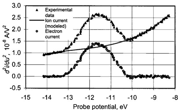
FIG. 1. High-energy part of the second derivative of the probe current. Neon pressure of 1.3 Torr. Discharge current of 20 mA, duration of 100 μs, and afterglow delay of 80 μs. The EEDF is calculated using Eq. (4).
