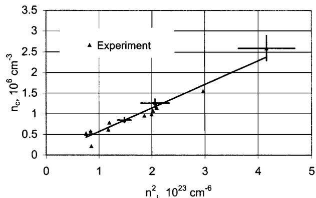
FIG. 3. Density of chemi-ionization electrons vs the squared combined density of  $1s_2$ ,  $1s_3$ ,  $1s_4$ , and  $1s_5$  states.
