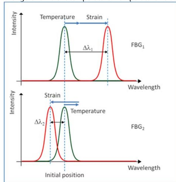
FBG spectrum shift due to physical stress and ambient temperature.
