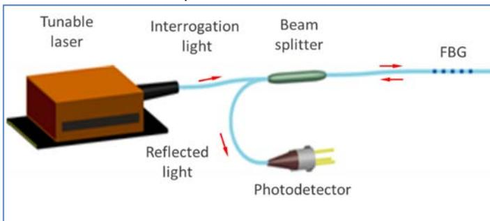
Instrumentation of the DFF sensor demonstrating the principle of the interrogation: a tunable laser that passes light into the fiber Bragg grating (FBG) through an optical circuit, which also detects the wavelength of the light reflected back by FBG.
