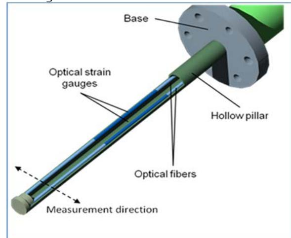
*A schematic diagram of the drag force flow (DFF) sensor showing internal structure of the hollow pin design. The deflection of the Fiber Bragg Gratings (FBGs) affixed on the inner surface of the pin (labeled as optical strain gauges) sensitively measures the force impact on the pin. Notice that the measurement direction of the flow force is along the imaginary plane that is formed by the two optical strain gauges.*
