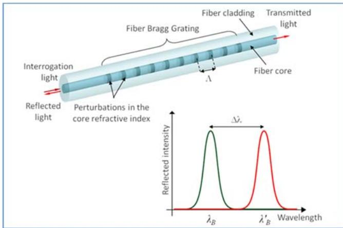
A detailed view of the fiber Bragg grating (FBG) as an optical strain gauge. Minuscule physical bending of the FBG leads to perturbations in the grating constant  $\Delta$  that impacts the characteristic wavelength of the reflected laser light. Measurement of shift in this wavelength,  $\Delta\lambda$ , is the core principle of DFF sensor's measurement of flow forces.
