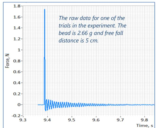
The pulse fall time is determined by the natural frequency of the probe oscillation. Applying the fast Fourier transformation (FFT) to the measured data shows a peak at 120.9 Hz (oscillation period of 8.2 ms). This is the natural frequency of the probe pin oscillation.
