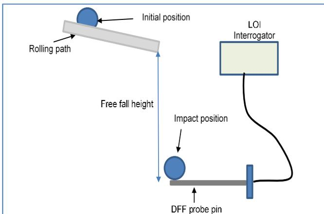
Polymer clay beads, density 1.38 g/cm<sup>3</sup>, were let to fall on the tip of a DFF sensor probe (type P-4000-40, rated
