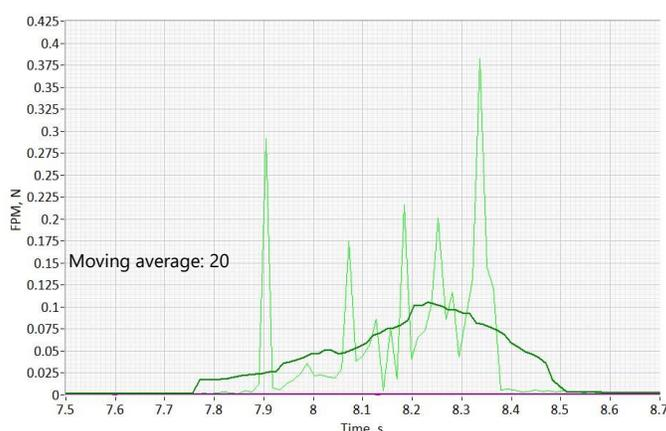
FPM moving average appears to be an appropriate metrics that differentiates the optimal mix from the under-processed powder. For moving average order 20, the value seems to increase steadily with time, reaching a maximum in about 0.5 seconds in both tests. The value of the maximum, or at any given time from the start of force action, for the optimal mix is approximately three times greater than that for the under-processed powder.
