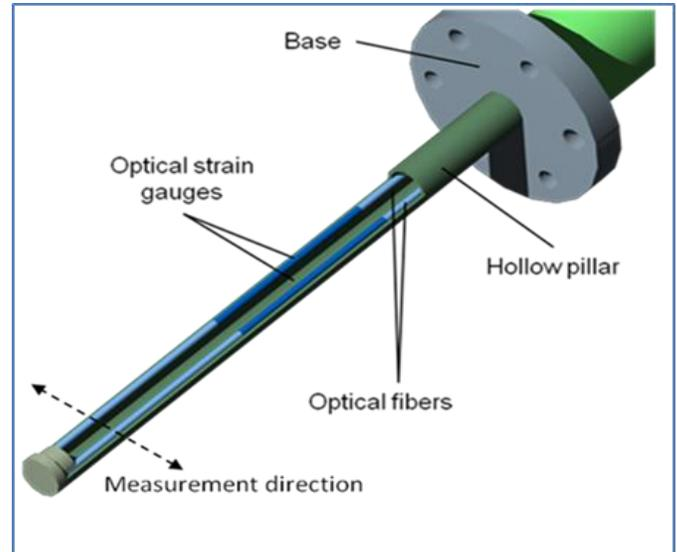
Employing optical sensing provides a number of advantages, such as the measurement is not affected by electromagnetic interference; the probe presents no ignition hazard, and the ability to withstand higher temperatures.
