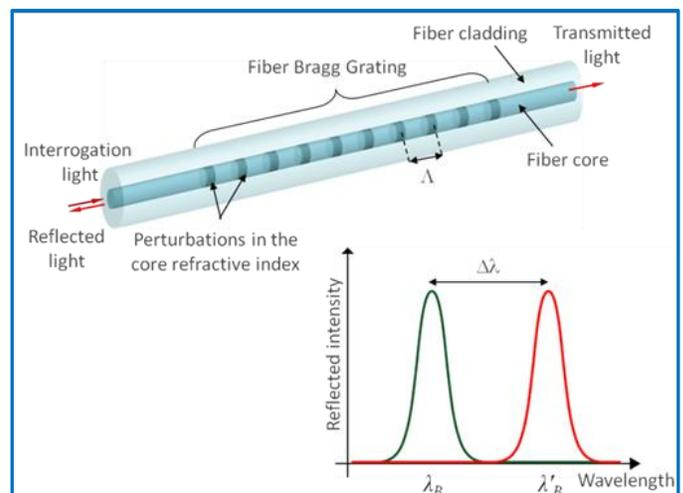
While being illuminated by broad-spectrum light, FBG reflects back only a portion of it that corresponds to a specific wavelength (green line spectrum). Bragg grating wavelength,  $\lambda_B$ , the center wavelength that is back-
