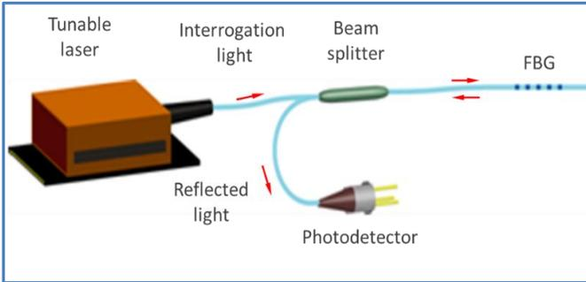
Measurement of shift in this wavelength,  $\Delta\lambda$ , is the core principle of DFF sensor's measurement of flow forces.
