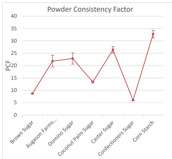
Figure 3. Powder Consistency Factor measured with the DFF Test Station. Error bars represent standard deviations over three tests. Brown, Coconut Palm and Confectioners sugar powders display lowest values of PCF which reflects their higher cohesiveness.
