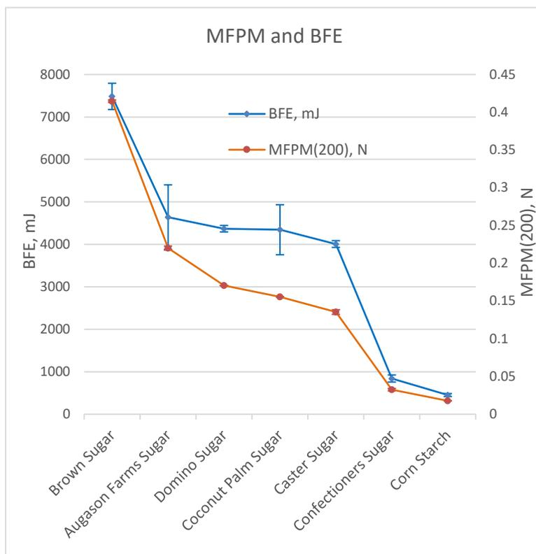
Figure 2. Comparison of BFE measured by FT4 and MFPM measured with the DFF test station. MFPM represents FPM averaged over 200 consecutive blades. See Appendix for more details of FT4 and DFF measurements. Error bars represent standard deviations over three tests.
