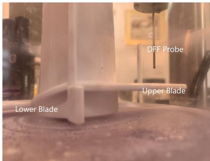
Figure 1. DFF probe inside the DFF Test Station mixer.
